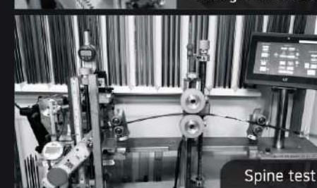
Straightness test
