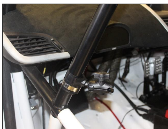
Here the 25mm rubber ball mount is securely attached to the A pillar bar of the roll cage.
