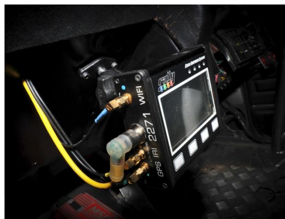
Here the 25mm rubber ball mount is securely attached to the A pillar bar of the roll cage.
