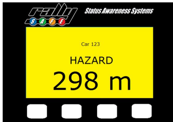
FIG 15: Warning - Vehicle is on or next to the road, status not yet confirmed [HAZARD]
