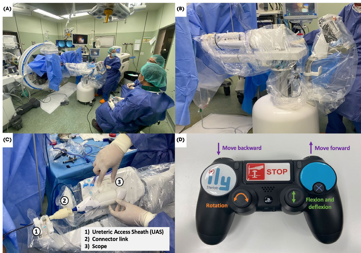
Fig. 1 (A, B) Operation room setting for roboRIRS with the ILY platform (STERLAB, Vallauris, France). The ILY robot is a compact trolley cart, weighing 40 kg. It is placed near the patient and remotely manipulated by the surgeon with a wireless controller, away from the ionising radiation source. (C) View of the ILY robot docking procedure: initially attached to the ureteric access sheath, then to the connector link, and finally to the scope. The undocking procedure is performed in the opposite direction. (D) ILY robot uses a wireless controller, similar to a video-game joystick, to remotely manipulate the flexible ureteroscope to perform the endourological movements. Arrows indicate hand movements to manipulate the scope. The ureteroscope can be moved forward and backward with the left and right frontal bottoms of the controller (purple arrows); and the flexion, deflection (green arrows), and rotation movements (orange arrows) with the right and the left joystick bottoms, respectively.
